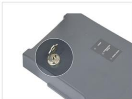
MCU W-2 locking position ON, joystick activated
